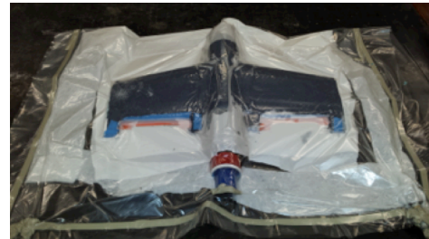
Figure 13. Vacuum Bag The vehicle in the process of being vacuum bagged while the composite wraps set
