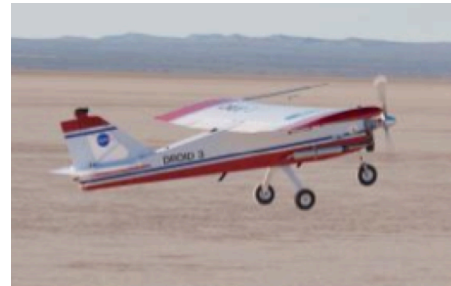
Figure 4. Example of a Conventional Aircraft Configuration NASA's DROID Flight Research Platform (Author's Personal Collection)
