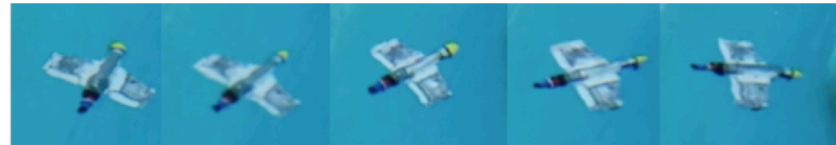
a) b) c) d) e) Figure 21. Vehicle Making a Right Turn During Testing Note the “slide” that occurs beginning between frames b) and c).
