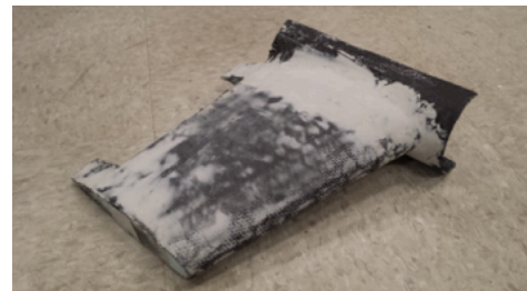
Figure 14. Wing The wing in its final constructed state. Black is the composite showing through the added white Bondo
